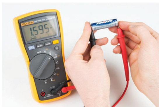
Figure 2.19 Measuring the emf of a cell
