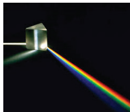
Figure 5.12 White light passed through prism – dispersion
