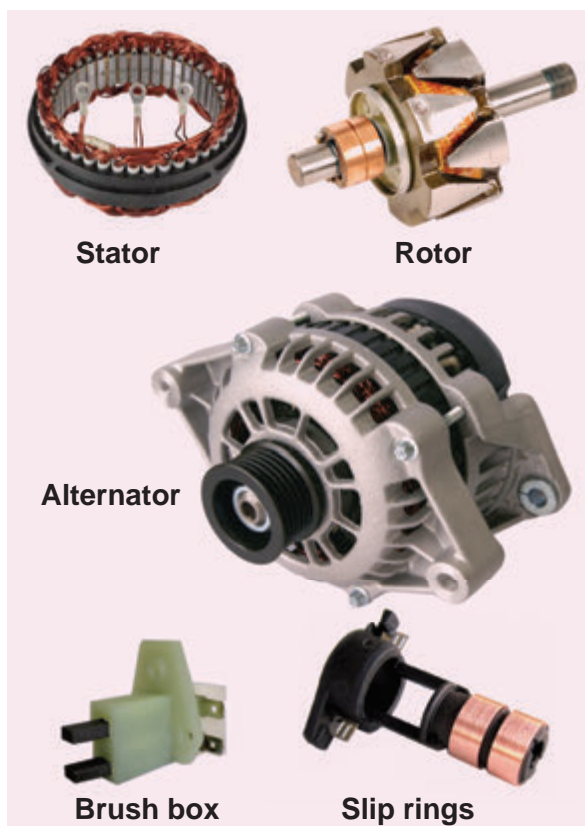
Figure 4.27 AC generator and its components
